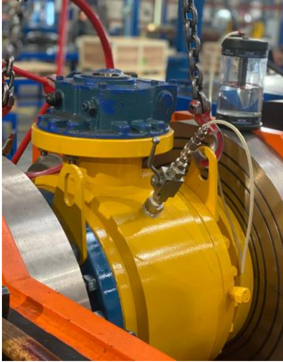
PNEUMATIC AIR TEST
